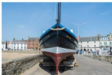
In the end the timber replaced was: the deck, the beams that hold up the deck, the stringer that holds up the beams, many of the timberheads which hold up the stringer, three outer planks and the bulwark, the heavy stroke, and the protective ironwork around the outside of the boat. She was refitted internally to match her original layout, and the engine was overhauled.
